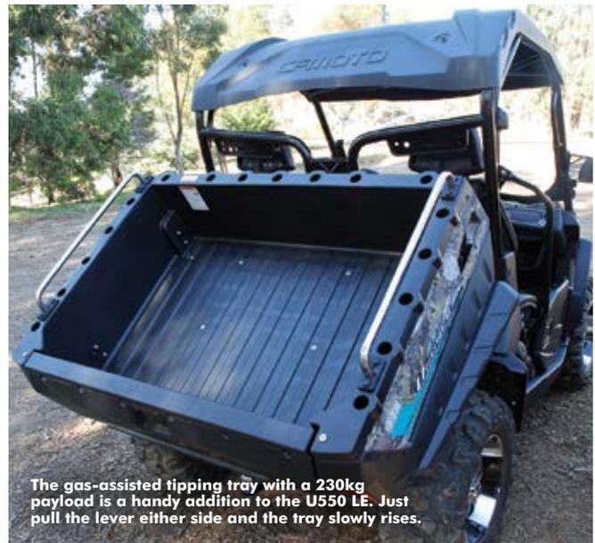
The gas-assisted tipping tray with a 230kg payload is a handy addition to the U550 LE. Just pull the lever either side and the tray slowly rises.
